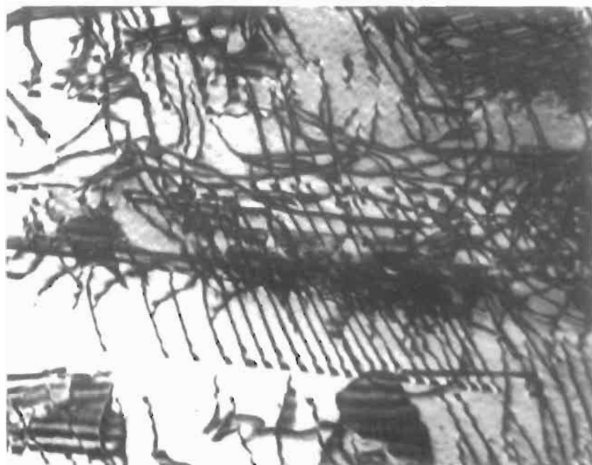
Fig. 4. Dislocations in Cu-10 at% Al single crystal foil deformed into stage II (from Howie [1960]). 23000 \times .
