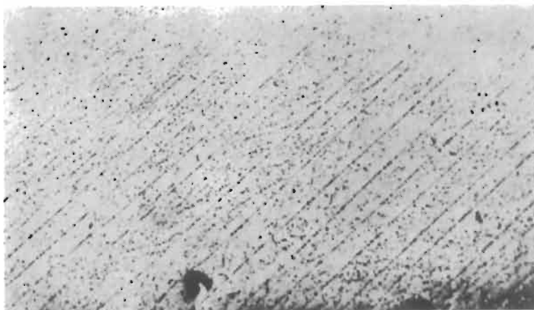
Fig. 9. Bent, annealed and etched single crystal of aluminum, showing sub-boundaries, 70 \times . (After CAHN [1949].)
