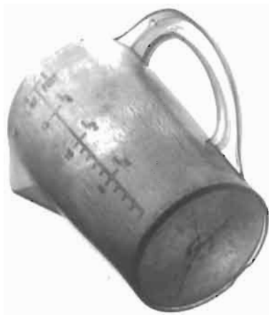
Fig. 34. Crazes in an injection-moulded polymer jug.
