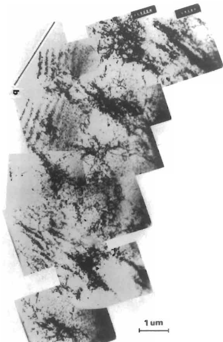
Fig. 9. Unit loop patches consisting almost exclusively of primary dislocations, seen on the primary glide plane for a stress of about 8 MPa. The direction of the primary Burgers vector, b , is indicated. This montage of micrographs was taken from a thin area of the foil as can be seen from the thickness fringes on the left side — the foil is wedge shaped and is tapering to a hole out of sight to the left. (Taken from BUCHINGER et al. [1986]).
